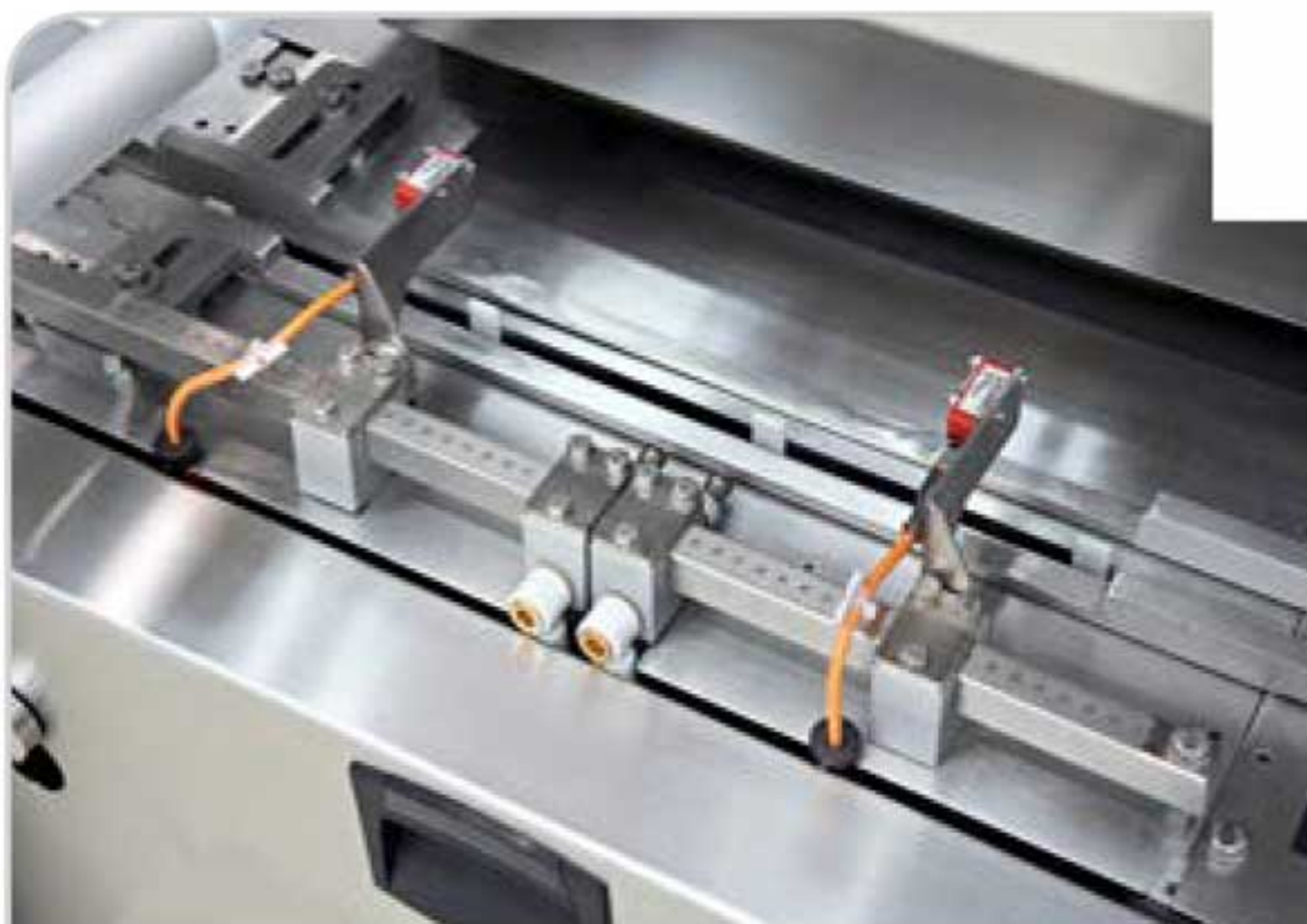
Misplaced product rejecter in the infeed conveyor
