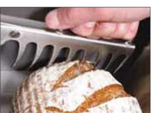
The gripper hook holds the loaf to be sliced securely and rigidly. The loaf's stability during the slicing process is a key requisite for a perfect result.
