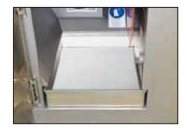
An easily removable tray successfully catches all the crumbs. This is assisted by guide plates etc. The crumb tray can be emptied and brushed out in no time. Bread cannot be sliced more hygienically than this.
