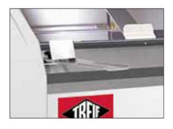
The bagging aid allows the cut loaf to be bagged easily.
