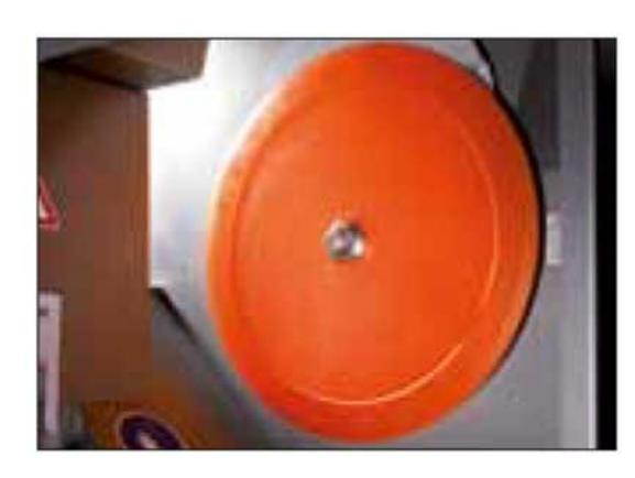
The Teflon-coated blade has unique toothing and a special grinding finish. Combined with planetary gearing, these features allow fresh bread to be sliced without blade lubrication.
