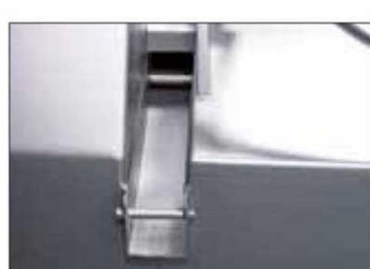
Cleaning channel for a better flow of liquids, e.g. rinsing water, and for blowing out of product rests.
