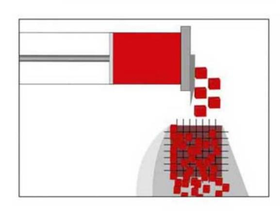
When dicing meat, the AVS (automatic pre-compression system) facilitates an optimum dimensional accuracy of the cubes and stripes right from the beginning.
