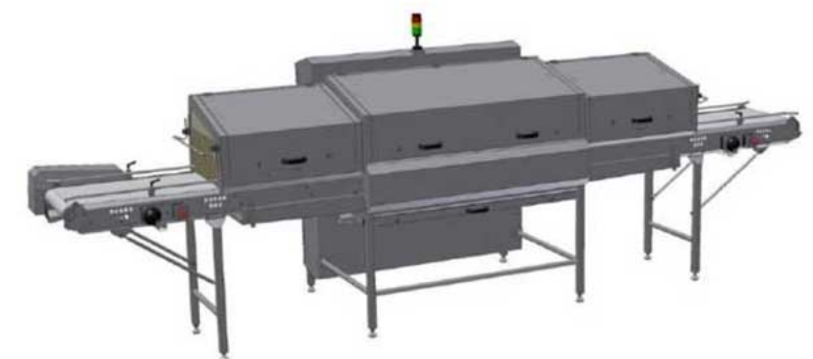
Example construction with inlet and outlet zone
